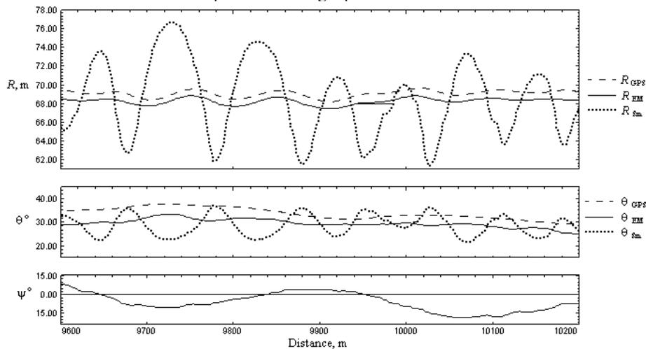
Fig. 10. Distance and angles measurements for Mi-8 helicopter.
