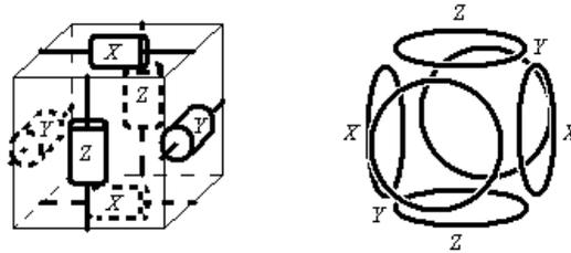
Fig. 2. EM-4H receiver (left) and GEOTEM receiver scheme (right).
