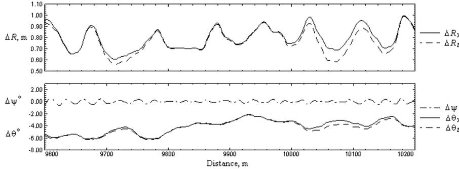
Fig. 11. Differences of the measured distances and angles for Mi-8 helicopter.
