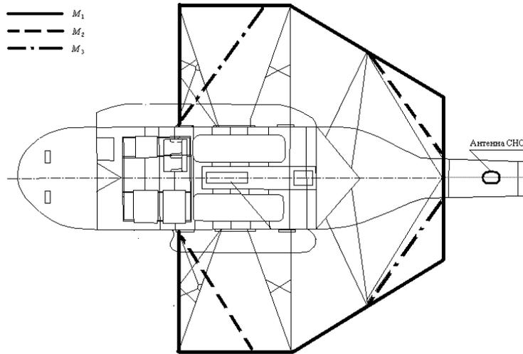
Fig. 8. Loops scheme for installation in Mi-8.
