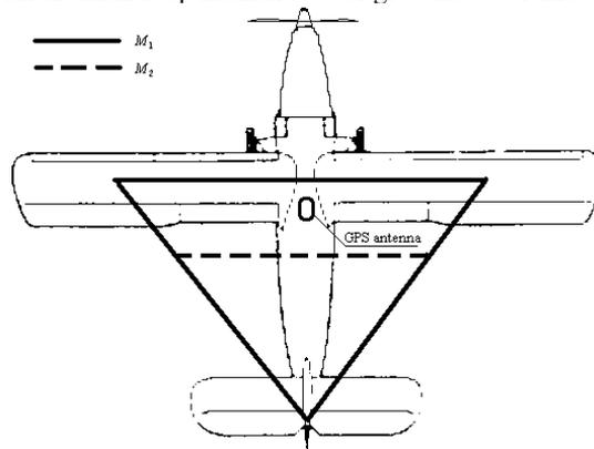
Fig. 7. Loops scheme for installation in An-3, An-2.
