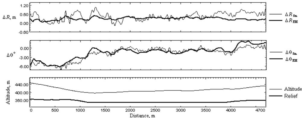
Fig. 12. Differences of the measured distances and angles for An-2 fixed-wing aircraft.
